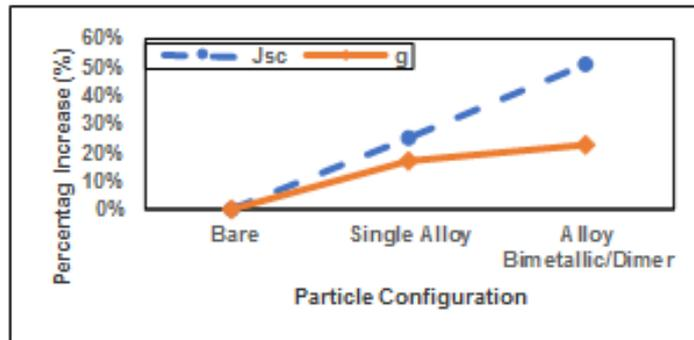
Fig. 7. Percentage change comparison for optical absorption enhancement factor ( $g$ ) and short circuit current density ( $J_{sc}$ ) for different nanoparticle configurations [14].
