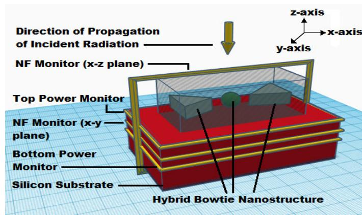
Fig. 8. Simulation setup for optical absorption enhancement and near-field analysis of the bow-tie hybrid nanostructure.
