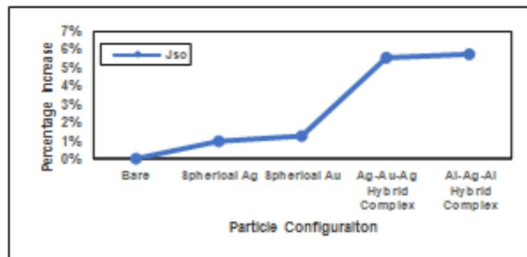
Fig. 9. Percentage change comparison for short-circuit current density ( $J_{sc}$ ) for different nanoparticle configurations [13].
