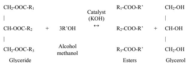
Transesterification is very rapid with alkali-catalyst compared to acid catalyst. Potassium hydroxide is used as catalyst to boost the reaction rate and biodiesel yield. Surplus methanol is applied to shift the reversible reaction to the product side.
